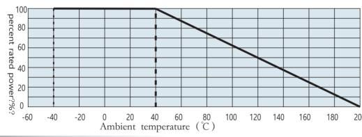
For resistors operated at an ambient temperature of 70°C or above, the power rating should be derated in accordance with the above derating curve.
